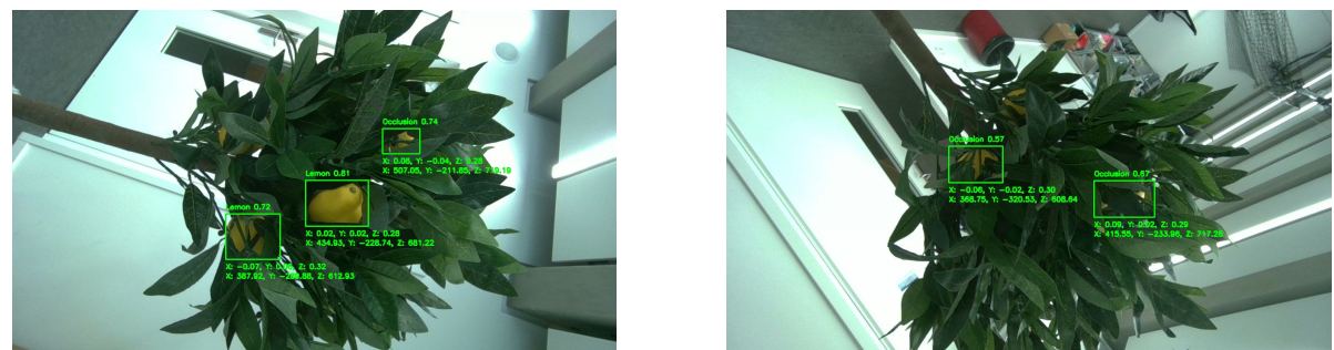
Figure 5.4: Successful detections of severely occluded fruits
