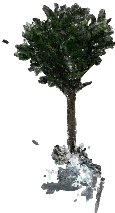
Figure 4.7: Finely filtered colored 3DGS point cloud
