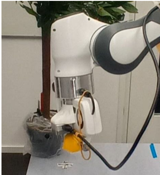
Figure 5.10: The only possible grasping direction on the Panda Hand gripper
