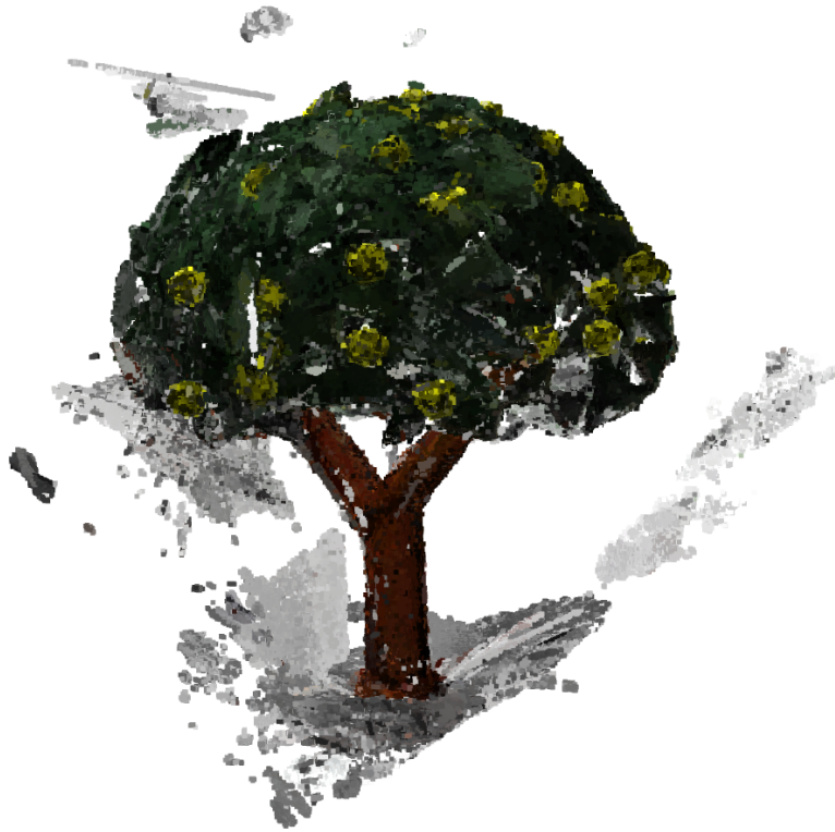
Figure 3.7: Finely filtered colored 3DGS point cloud
