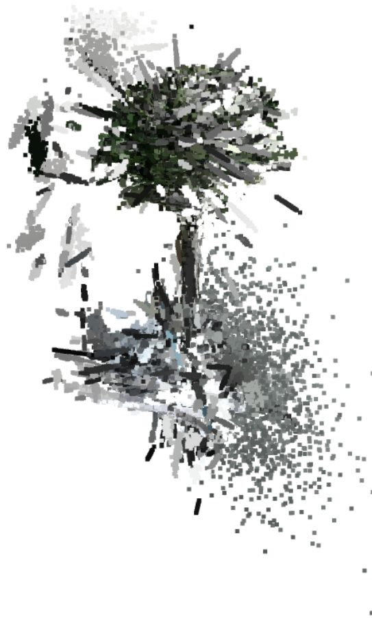
Figure 4.6: Coarsely filtered colored 3DGS point cloud
